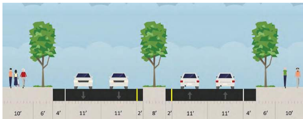
Image 22 – Proposed Roadway Typical Section between the Connecticut College Main Entrance and Deshon Street
