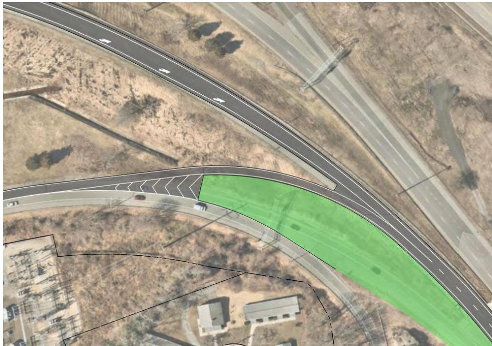
Image 24 - Realigned Exit Ramp
