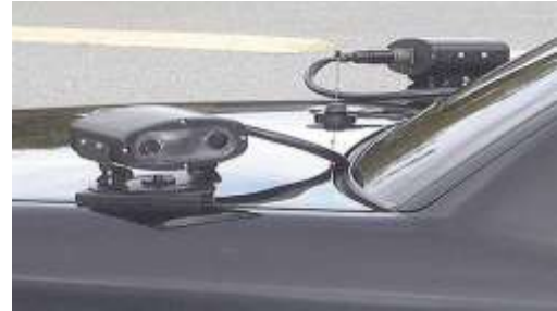
Figure 5: Sample LPR Installation
