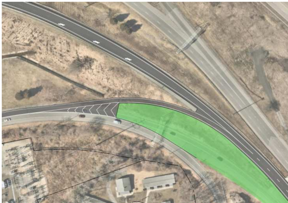
Image 24 - Realigned Exit Ramp
