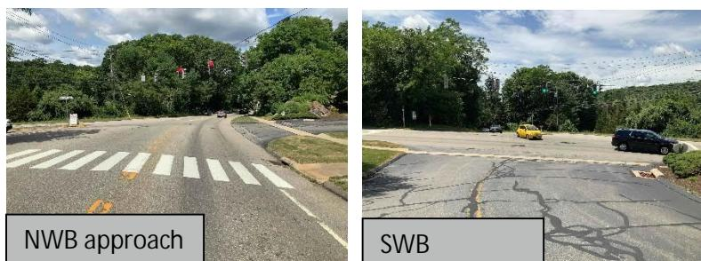
Chapman Farms Road has one undesignated approach lane and one departure lane. The traffic signal at this intersection is uncoordinated and operates on a single controller with the signal at the intersection of Route 161 and Roxbury Road. A crosswalk is located on the south leg of the intersection.
