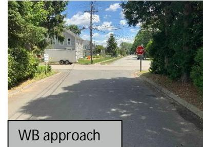
Route 161 (Pennsylvania Avenue) and Hope Street is an unsignalized T-intersection. Hope Street is Stop controlled with a one lane approach. Route 161 is uncontrolled and has one approach and departure lane in each direction. There is a crosswalk across the southern leg of Route 161.
